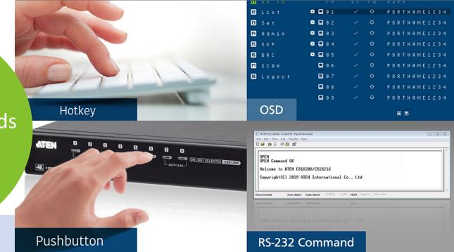
Port switching is as easy and convenient as pressing the front-panel pushbuttons, pressing supported hotkeys, using the OSD, or entering RS-232 commands, whichever works best for you.
