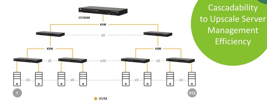
By connecting computers to a 4K USB 3.0 Rack KVM Switch, the number of connected computers can be scaled up to 256 by cascading the CS19216 in 2 levels, or 512 by cascading the CS18208 in 3 levels, leaving room and flexibility for network expansion when needed.
