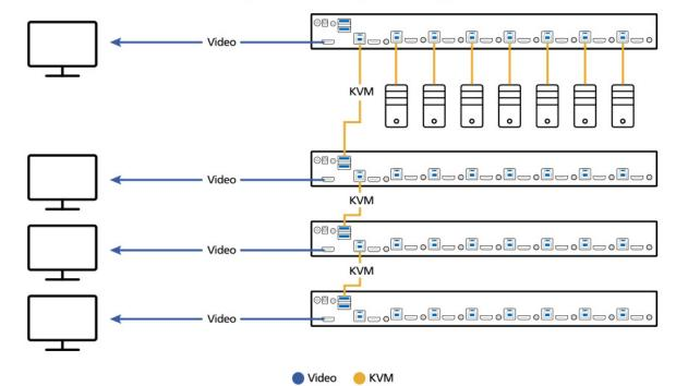
When a large amount of complex content needs to be viewed at once or there's a need to examine intensive data for analysis, up to 8 Rack KVM Switches can be stacked up to allow up to 8 monitors to be set up in a multi-display configuration (such as dual- / triple- / quad-display) to facilitate live feeds among computers at the console desktop.
